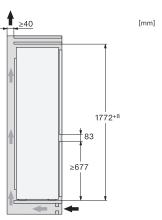
KD7713E Active, KDN7713E Active, side view (installation drawings)
