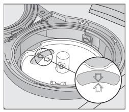
Put the holder back into place so that the arrows in the PowerDisk holder and in the viewing window point towards each other. The holder must lie flat. The AutoDos lid must close tightly so that the detergent powder does not get wet and clump together. Make sure that all seals are clean.
